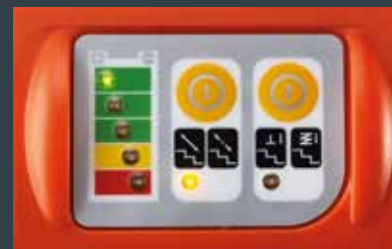
Battery display, single step control and ComfortStep
